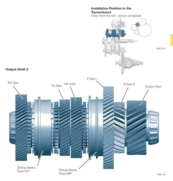
The following are located on output shaft 2:
