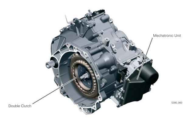
The dry double clutch has an extensive impact on the entire transmission concept. In comparison with the directshift transmission 02E, efficiency has been considerably improved. This improved efficiency makes a significant contribution towards lowering consumption and emissions.
