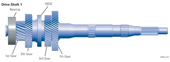
Drive shaft 1 is connected to clutch K1 via splines. It is used to shift gears 1, 3, 5 and 7. To record the transmission input speed, this shaft has the impulse wheel for G632 Transmission Input Speed Sensor 1.
