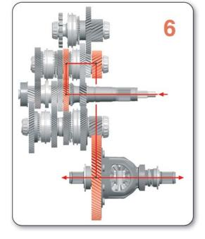
6th Gear Clutch K2 Drive Shaft 2 Output Shaft 2 . Differential
