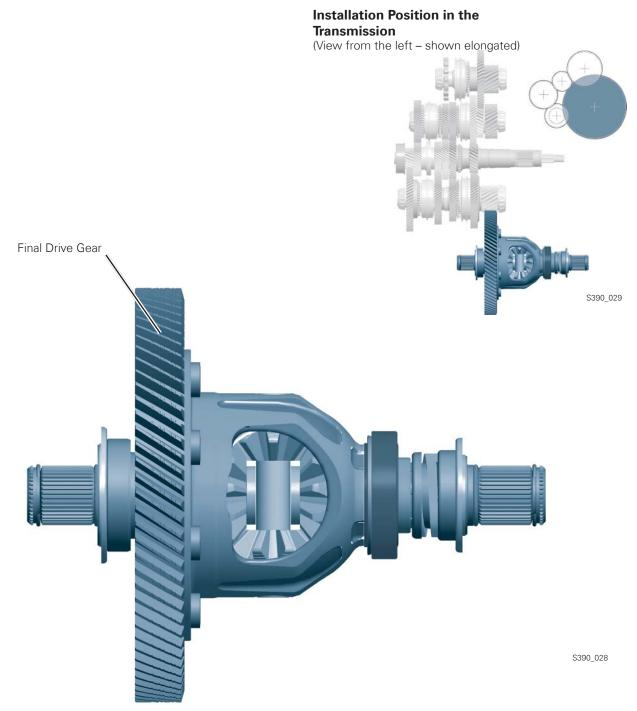
The differential transfers the torque onwards to the vehicle wheels via the drive shafts.
