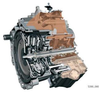
Mechatronic Module Oil Circuit for Mechanical Transmission
