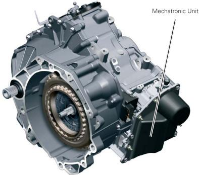
The electornic control unit is the central transmission control unit. All sensor signals and all signals from other control units come together here, and all actions are performed and monitored by it. Eleven sensors are integrated into the electronic control unit; only the G182 Transmission Input Speed Sensor is located outside of the control unit. The electronic control unit hydraulically controls and regulates eight solenoid valves for shifting the seven gears and for actuating the clutch.
