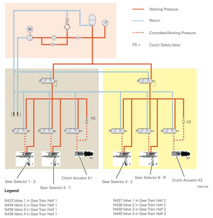
The clutch safety valves enable the clutches to be drained and therefore opened in the event of a fault.
